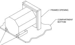
SECURE CHOCKS, ONE ON EACH SIDE, TIGHTLY AGAINST WATER HEATER JACKET AND FASTEN TO VEHICLE FLOOR TO PREVENT MOVEMENT. CHOCKS SHOULD BE APPROXIMATELY 2" X 2" X 6"
